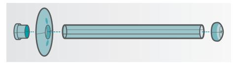
Assemble the drying stand as shown by inserting the tube through the disc, then onto the base. Finally, place the cap on top of the tube. The drying stand may be shortened by trimming the tube before placing onto the
