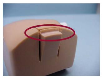
Battery latch height adjustment
