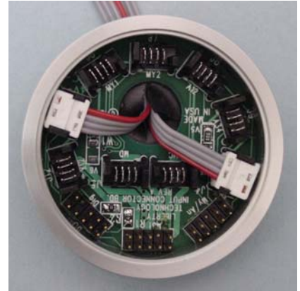
Fig 12. Two dual-action switches. Use D12, D34.
