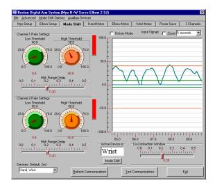
2) These levels are adjusted by rotating the *Low Threshold* (green) and *High Threshold* level (orange) knobs. The corresponding line on the graph will change accordingly (see screen to the right).
