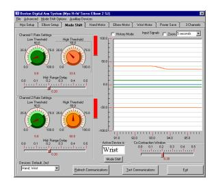
3) Once the threshold levels are properly adjusted, the patient should be able to repeatedly make strong, rapid contractions and exceed the *High Threshold* level (as shown on the screen to the right).
