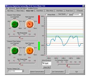
7) Once both channels have been set up independently, they must be tested together. To do this, have the patient contract both muscles simultaneously. Both green bars should illuminate and the *Active Device* window should display a different device (i.e. hand, wrist).
