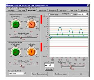
4) If the patient can repeatedly make strong muscle contractions and exceed the *High Threshold* level, but the red bar does not turn green (indicating a successful rapid contraction), then they are not providing the signal rapidly enough. To accommodate them, you must increase the time allowed to achieve this. This is done by adjusting the *Co-Contraction Window*, sliding the lever to the right. Repeat this process until
