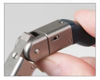
Apply pressure to the back of the fingertip, which causes the fingertip to ratchet into flexion. Once the desired position is determined, pressure can be removed from the fingertip and the tip would be locked in to position.
