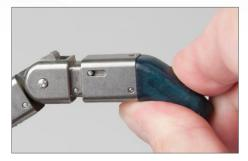
To return the fingertip back to the extended position, dislocate the tip section from the base by pulling on the tip section. This motion releases a pin in the tip section from the base allowing the finger to move freely. Once the desired position is determined, the pull on the fingertip can be released and the finger will engage in the new locked position.
