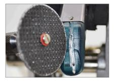
Secure finger and using a dremel tool cut a channel down the length of the tip. Take caution to not cut in to titanium.
