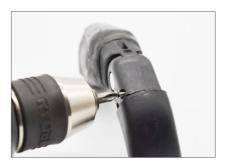
Insert long 0-80 screw to secure spring into fingertip. Tighten with small Phillips screwdriver.
