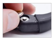
Insert retaining ring. Only install retaining ring at final assembly.
