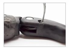
Insert both ends of cable through hole in fingertip and exit through the bottom. The photo on shows the 2 cables converting into one as they pass through the cable cleat. Both cables go through the finger base
