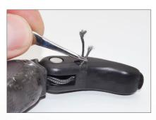
Pull both ends through bottom slot on finger base with tweezers and exit through threaded hole on side of fingertip. The cable cleat allows the two cables to come together; both cables follow the same line through the process and exit out of the finger together
