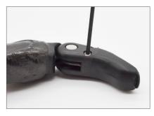
Install Allen screw to secure knot in place. Do not overtighten.
