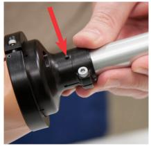
9. Once final alignment is set. Drill .125 hole through the hole in the bottom tube clamp.
