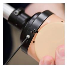
**8.** Tighten screw on clamp ring. Do not overtighten. Recommended torque 4.5 in lbs (.5n/M). Lighter torque is acceptable to allow friction movement.
