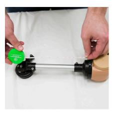
**4.** Determine length of 20mm tube and cut tube to desired length and reassemble
