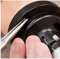
7. Determine best location for rotation limit pins (.060x.187) and Insert the roll pins into desired holes around the circumference of the Boston Arm Adapter. The rotation limit can be set between 90-270°
