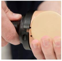
2. Remove screw of the Bottom clamp ring
