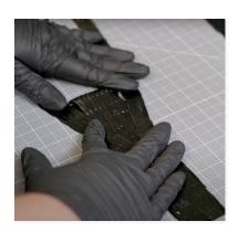
The College Park Intelliweave composite technology is a proprietary process developed to bring the maximum amount of strength and flexibility to a prosthetic foot. Unlike the standard carbon fiber 2D layering process, Intelliweave allows for unlimited 3D woven patterns and complete control of the exact areas that need strength and those that need flexibility.
