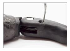
Insert both ends of cable through hole in fingertip and exit through the bottom. The photo on shows the 2 cables converting into one as they pass through the cable cleat. Both cables go through the finger base
