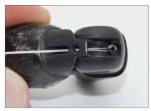
Insert thread through spring loop and pull through with tweezers then exit both ends of thread through oval slot on finger base. The two threads will be close together in order to get them through the oval slot in base. Apply tension until you see the spring loop. Insert short 0-80 screw into hole on finger base and secure screw and spring with Phillips screwdriver. Remove thread
