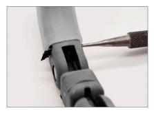
Push out knot from 1/16" hole on opposite side with supplied 1/16" rod.
