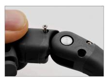
Apply tension to pull spring loop back to screw hole. Once you see the spring loop through the screw hole insert Long 0-80 screw to lock spring in place. Tighten screw with Phillips screwdriver and remove thread
