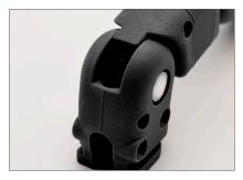
Install base spring. Align spring loop with screw hole, insert 0-80 screw and tighten with Phillips screwdriver to lock spring in place.
