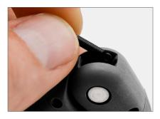
Install spring into tip as shown.
