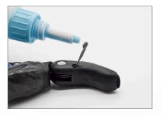
Silicone wrist band fabricated at fabrication center should be placed over apex of knuckle. Pull both cables exiting finger to proper length and knot. Have patient flex and extend finger to make sure cable length is set to their preference. Superglue knot, Let superglue set then pull knot into hole.
