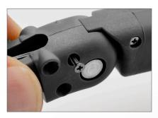
Apply tension to pull spring loop back to screw hole. Once you see the spring loop through the screw hole insert 0-80 screw to lock spring in place. Tighten screw with Phillips screwdriver and remove thread.
