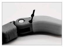
Tie new knot and apply super glue to back side of knot. Cut cable 1/8" past knot.
