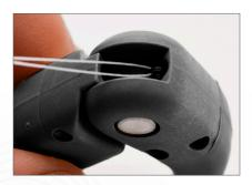
Insert thread through exposed spring loop and pull through with tweezers.
